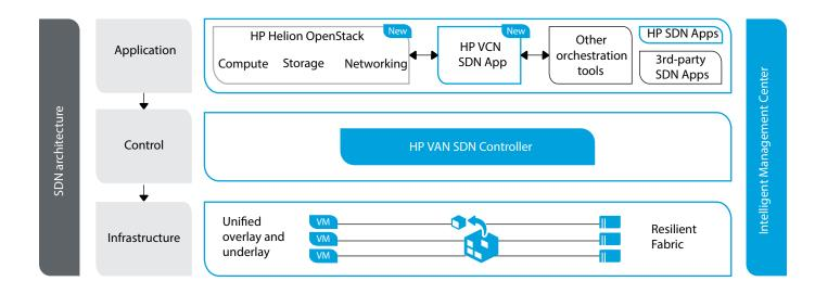
VCN is bundled with HP Helion OpenStack Neutron, which has unique HP enhancements, including distributed virtual routing (DVR), multi-hypervisor support, high availability, a VXLAN gateway, VPN and security group enhancements, and improved scalability. DVR, for example, optimizes and improves the scale of connections by supporting direct connectivity among different NV switches (VNS) as well as connectivity between virtual hosts and the external network.
