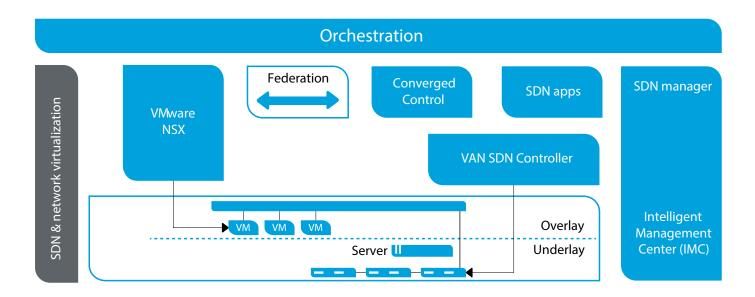
The HP VAN SDN Controller supports both the KVM and ESXi hypervisors, and federates the VAN controller and the VMware NSX network virtualization platform through federation APIs. NSX communicates with the VAN controller using the Open vSwitch database (OVSDB) management protocol. OVSDB is used to manage Open vSwitch instances, and manipulates a set of tables representing switch configuration data.
